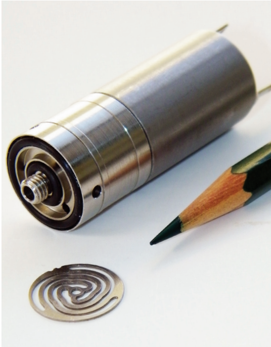
The spider spring shifts the valve when the solenoid de-energizes and has a stroke of only 0.018 in.
